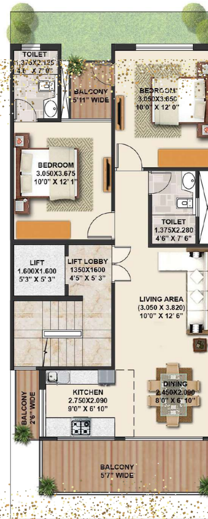
TYPICAL FLOOR (1ST, 2ND, 3RD & 4TH)
